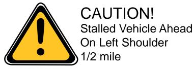
A TMC operator will use the SunGuide software to generate a traveler advisory message (TAM) to broadcast to equipped vehicles in the vicinity-specific region. The OBE user interface displays this message to drivers.
